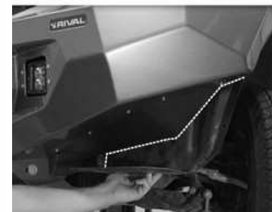
47. Install mudguards onto the vehicle and mark the cutting line.
