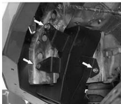
40. Install the washer reservoir using the bracket and standard fittings.
