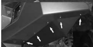
45. Install the flaps onto the vehicle using screws M6x20
