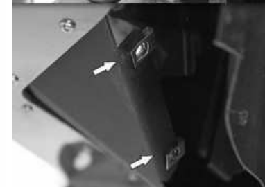
50. Install caged nuts onto the flap.
