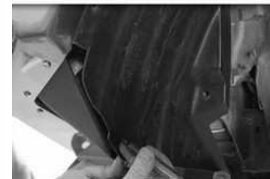
49. Install the mudguard onto the vehicle, mark drilling points opposite the holes of the flap and drill the flap holes.
